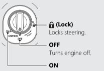
Turns electrical system on for starting/riding.
