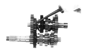
Install the mainshaft and countershaft into the left crankcase.
