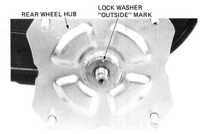
Tighten the rear axle nuts.
