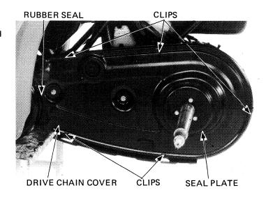
Apply grease to the splines on both end of the axle.
