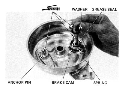
Insert the end of the spring into the hole in the brake cam.
