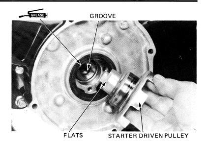
Install the pulley bolt, washer and O-ring.
