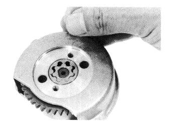
Measure the pump tip clearance.
