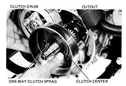
Install clutch plate B onto the clutch drum.
