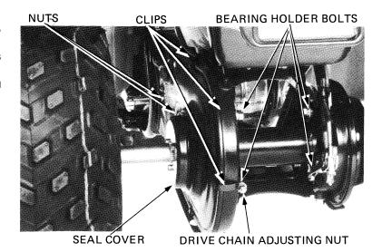
Remove the drive chain master link clip, master link and drive chain.
