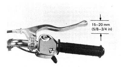
Adjust free play by turning the adjusting nut.
