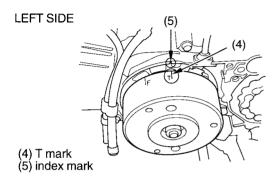
3. Rotate the generator flywheel counterclockwise until the T mark (4) on the flywheel lines up with the index mark (5) on the crankcase. In this position, the piston may either be on the compression or exhaust stroke.
