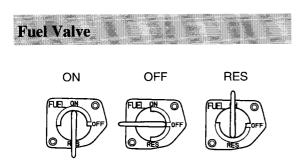
The three-way fuel valve is used to control the flow of fuel from the fuel tank to the carburetor.
