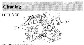
(1) attaching screws(2) air cleaner housing cover
