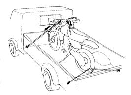
To secure your motorcycle, brace the front wheel against the front of the truck bed or trailer rail. Attach the lower ends of two straps to the tie-down hooks on your vehicle. Attach the upper ends of the straps to the handlebar (one on the right side, the
