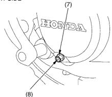
(7) clutch lock nut(8) clutch adjuster
