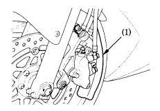
3. Remove the socket bolt A (2) and socket bolt B (3).
