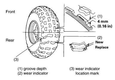
To check the condition of a tyre tread, measure the groove depth (1) in the centre of the tyre, or check the wear indicator (2).
