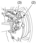
(2) brake lever adjusting nut(3) brake arm pin
