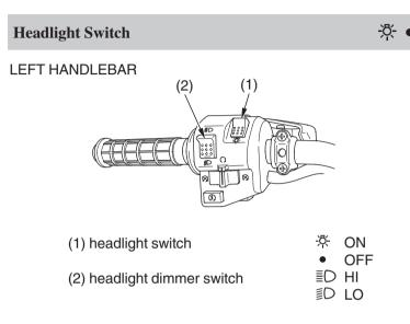
The headlight switch (1) is used to turn the headlights and assist headlight ON (  $\stackrel{\infty}{\rightarrow}$  ) or OFF ( • ). To operate, turn the switch to ON (  $\stackrel{\infty}{\rightarrow}$  ) or OFF ( • ).
