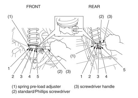
The spring pre-load adjuster (1) has 5 positions for different load or riding conditions.
