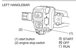
The start button (1) is used for starting the engine. Pushing the button in starts the engine. See Starting Procedure, page 113.
