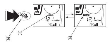
To reset the tripmeter to zero, press and hold the odometer/tripmeter select button for more than 2 seconds.
