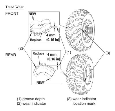
To check the condition of a tyre tread, measure the groove depth (1) in the centre of the tyre, or check the wear indicator (2).
