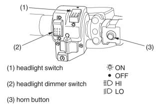
The headlight switch (1) is used to turn the headlight ON (  $\stackrel{\star}{\leftarrow}$  ) or OFF ( • ). To operate, turn the switch to ON (  $\stackrel{\star}{\leftarrow}$  ) or OFF ( • ).
