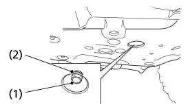
(1) engine oil drain bolt
