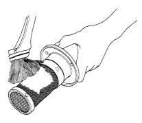
4. Install the spark arrester and the gasket in the muffler and tighten the three bolts securely.
