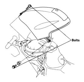
Front Lower Cover Remove the bolts, then slide the cover forward.
