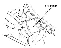
3. Apply a thin coat of engine oil to the rubber seal on the new oil filter.
