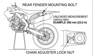
3. Measure the *loaded with rider* dimension. Remove the workstand. With two helpers available, sit as far forward as possible on your CRF's seat, wearing your riding apparel. Ask one helper to steady your CRF perfectly upright so you can put both feet on the pegs. Bounce your weight on the seat a couple of times to help the suspension overcome any situation and settle to a good reference point. Ask the other helper to measure the *loaded* with rider dimension.
