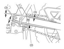
5. Measure a section of the drive chain to determine whether the chain is worn beyond its service limit. Remove the drive chain and measure the distance between a span of pins from pin centre to pin centre. If the distance exceeds the service limit, the chain is worn out and should be replaced.
