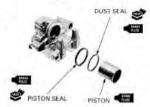
If the caliper and bracket pin boots are hard or deteriorated, replace them with new ones.
