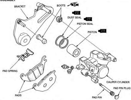
Coat the new piston seal and dust seal with clean brake fluid and install them in the seal grooves of the caliper.
