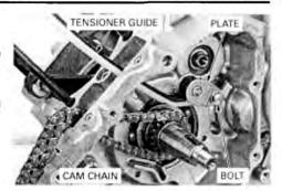
Remove the circlip, washer, spring and bearing push plug from the left crankcase.
