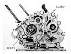
Remove the right crankcase bolts and washer.
