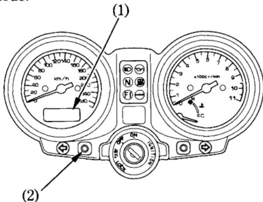
(1) Odometer/Tripmeter display
