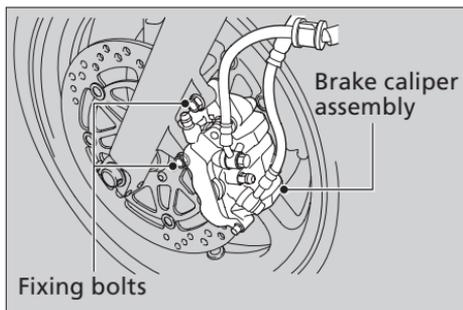
3. Remove the right and left caliper assemblies from the fork leg by removing the fixing bolts.
