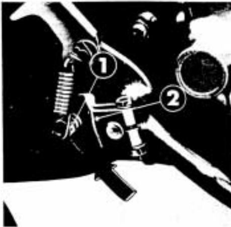
① Nut ② Chain tensioner plate
