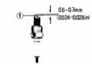
(1) Bend side electrode to adjust gap
