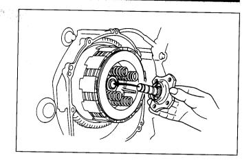
Secure the lifter plate by tightening the bolts in crisscross pattern in several steps.
