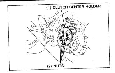
Temporarily remove the tool and tighten the nuts, then reinstall the clutch center holder onto the bosses of the pressure plate.
