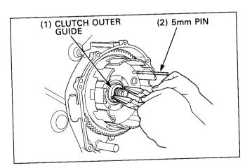
Align the projections of the crankcase with between the teeth of the primary driven gears and remove the clutch outer from the mainshaft.
