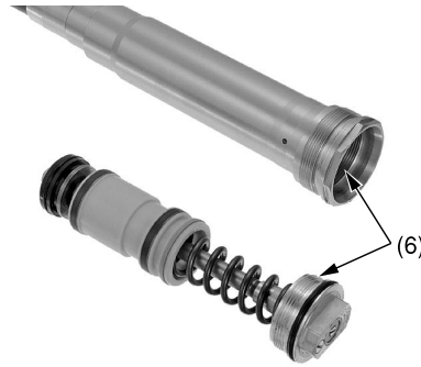
(6) fork cap and fork damper threads
