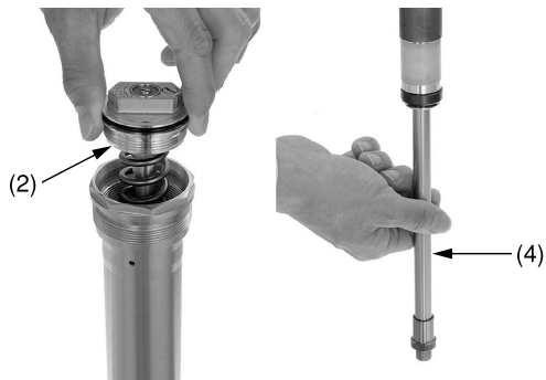
(2) fork cap assembly (4) fork damper piston rod
