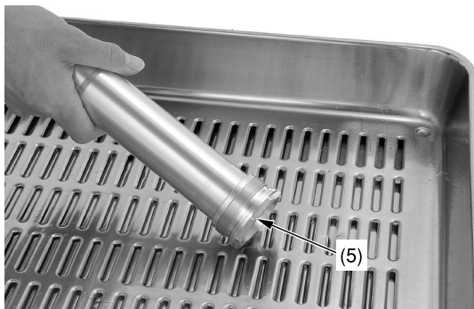
(5) fork damper oil/spring chamber
